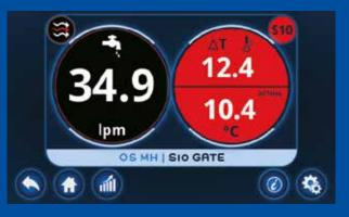
By clicking on a specific circuit you will see detailed information, including delta T (heat transfer) of the specific channel. Also, turbulent flow indicator is included.
