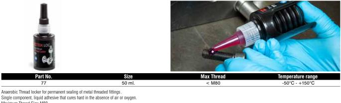
Single component, liquid adhesive that cures hard in the absence of air or oxygen. Maximum Thread Size: M80. Disassembly strength: High. Temperature range: -50°C - +150°C. Breakaway torque: 32 Nm. Pack sizes: 50ml.
