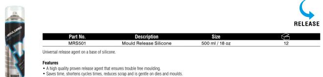
Suitable for thermoplastic or thermoset moulding
