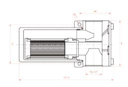
Dirt particles in coolants often result in blockages in small cooling channels and can render mould inserts useless. This maintenance friendly Mould-pro stainless steel in-line filter MPF-80-200 offers superior low cost protection against foreign body particles, in particular for conformal cooling channel of injection moulding tools.
