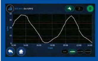
Data i stored in the internal memory and can be displayed in graphical view for each circuit. Data can also be exported for external use.
