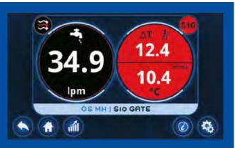
By clicking on a specific circuit you will see detailed information, including delta T (heat transfer) of the specific channel. Also, turbulent flow indicator is included.
