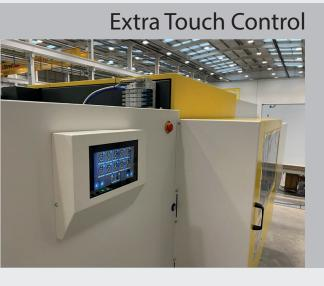
Flosense is designed to operate with an extra touch screen on non-operator side of easy acces when controlling cooling lines installed remotely.
