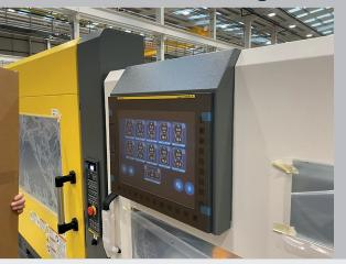
Flosense installed on the Fanuc Machine Control. The integration is made using VNC technology allowing to operate the full Flosense GUI directly on the Fanuc Touch Control.
